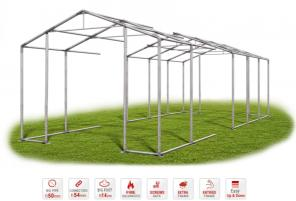
Main construction is based on steel tubes ab. Ø 50mm and connectors ab. Ø 54mm. galvanized construction. Through and through screws guarantee reliable connection. The Easy Up & Down System allows a quick change of the tent's height.
