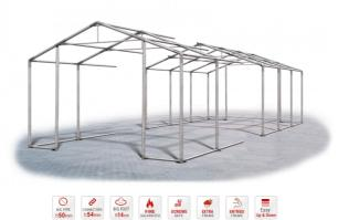
Main construction is based on steel tubes ab. Ø 50mm and connectors ab. Ø 54mm. galvanized construction. Through and through screws guarantee reliable connection. The Easy Up & Down System allows a quick change of the tent's height.
