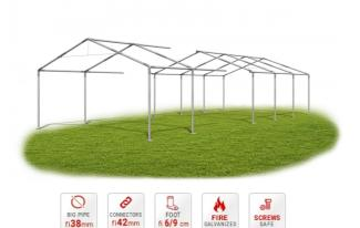
Main construction is based on steel tubes ab. Ø 38mm and connectors ab. Ø 42mm. galvanized construction. Through and through screws guarantee reliable connection. Feet of the marquee: 6 by 9 cm.
